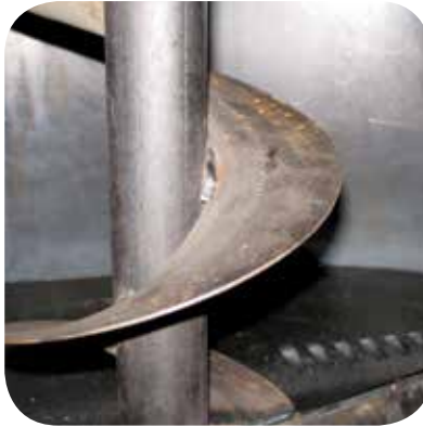
Auger/ Agitator ensures even mixing and eliminates temperature stratification.
